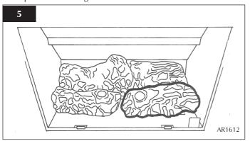
5.4 Place log D across from the rear log A to log B on the left-hand side. There are cut-outs in both logs for location. See diagram 6.
